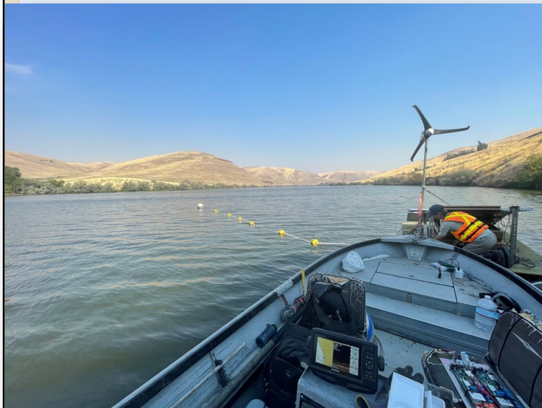
Above: Floating PIT antenna barge at the 2022 location, slightly upstream from Phillipi Campground. Small wind turbine attachments were added in addition to the solar panels for supplying sufficient power to the antennas. - ODFW
