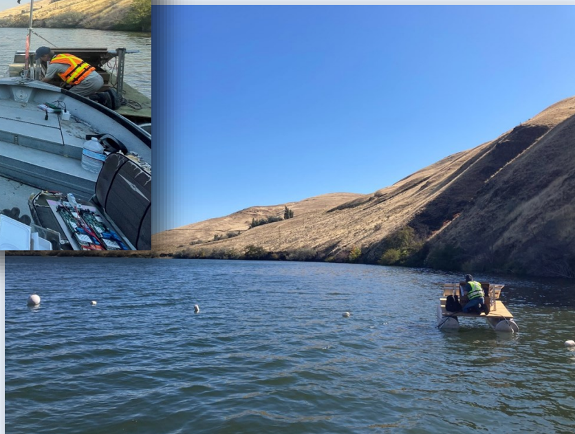
Above: Floating PIT antenna barge at the 2022 location, slightly upstream from Phillipi Campground. Small wind turbine attachments were added in addition to the solar panels for supplying sufficient power to the antennas. - ODFW
